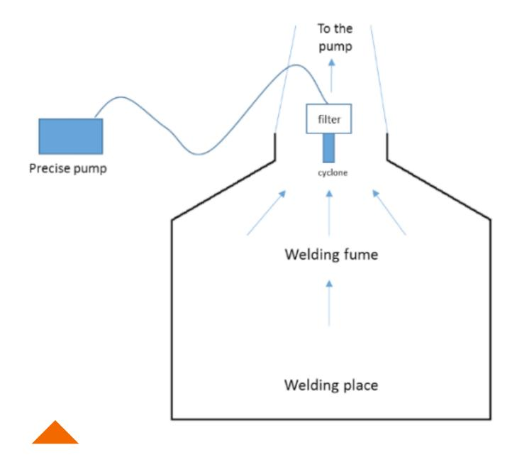
Figure 1. Schematic view of welding chamber for manganese exposure measurement.
